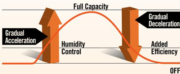
Gradual acceleration and deceleration of the variable speed motor significantly reduce sound.
